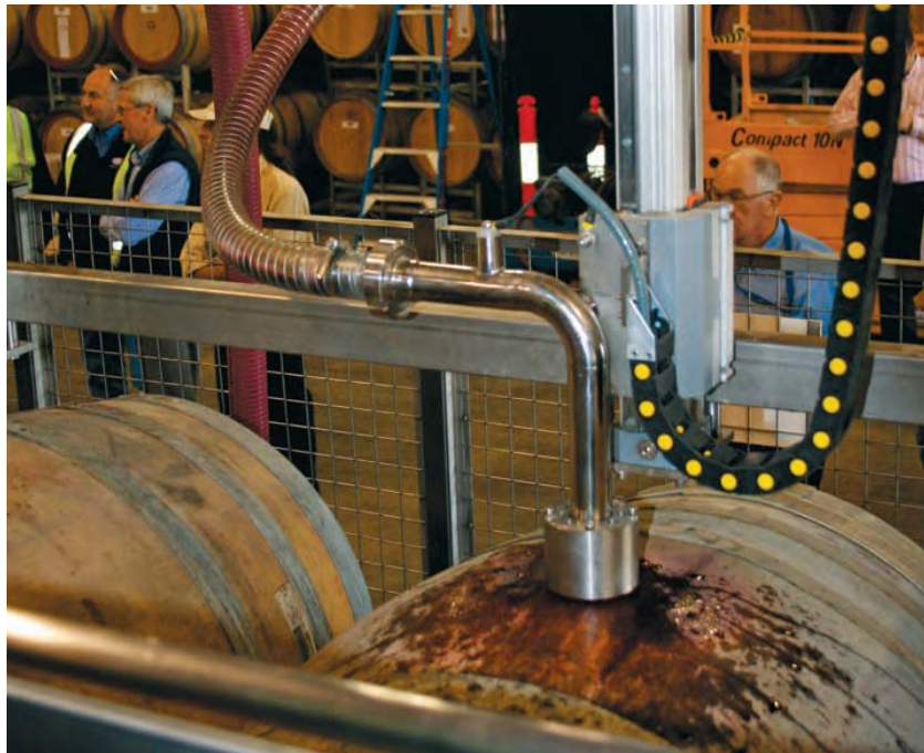
The EKINSA automated system pumping out the wine.
