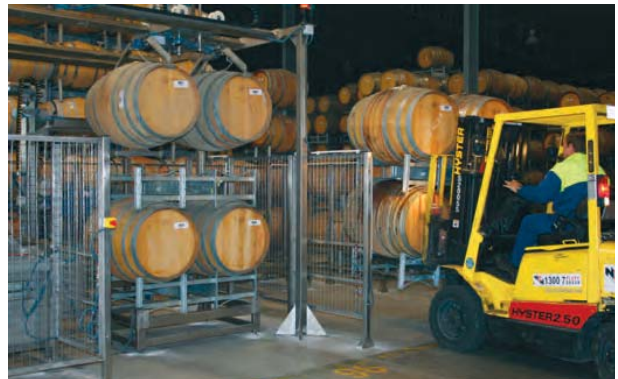
The forklift driver loads the wine barrels onto the crate ready for the machine to pick up.
