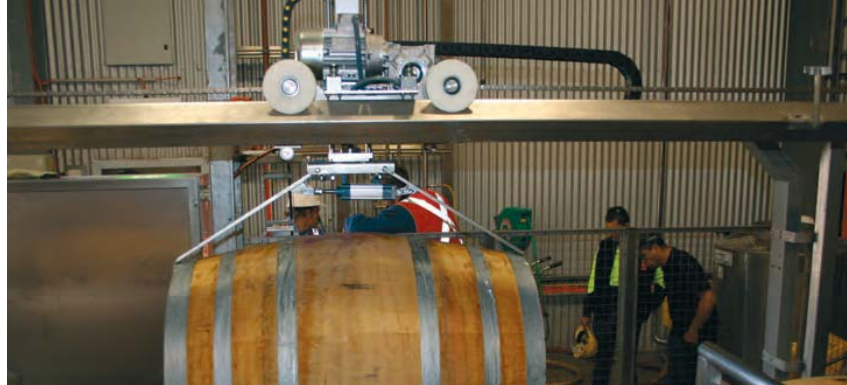
The EKINSA automated system takes the empty barrels across the machine to be filled.
