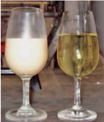
Compare the difference. Left: Sample Viognier from tank. Right: post-filter. Samples taken at the same time.
