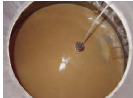
Residue in tank at completion of filtration of Viognier wine. Photo taken through expansion chamber of tank.
