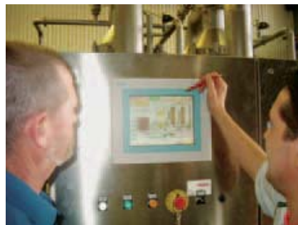
A touch screen offers a simple way of staying in control of filtration processes.
